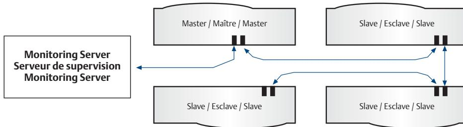
A connecting cable between the unit controllers creates the LON via which communication takes place between all units in a network.
